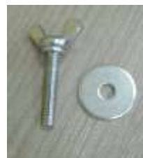
Fig.3: Screw for supporting the bracket on the appliance
